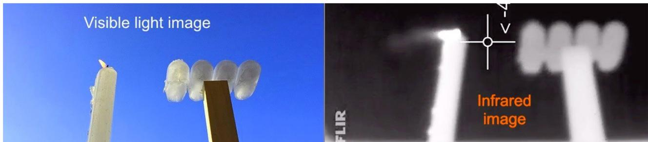
Looking up at a platform holding a lit candle and ice on a pedestal, a typical thermal imaging camera shows that the ice is appreciably warmer than the clear blue background sky. Assuming a 0.95 emissivity, ice at 0°C would be radiating about 299.88 watts per square meter. This means that a typical thermal imaging camera is capable of detecting 300 W/m<sup>2</sup> of thermal radiation.
