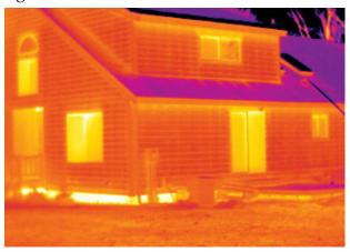
Thermal IR image of a house, showing IR radiation passing straight through the glass windows.
